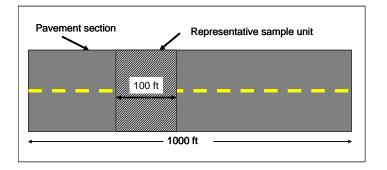
The area of AC sample units should be 2500±1500 square feet, and for PCC sample units, this should be 20±8 slabs. The total inspected area or slabs for a pavement section must be at least 10% of the total pavement section area or slabs. <u>This is an exception to the</u> procedure described in ASTM D6433.
